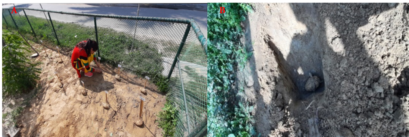
Figure 1: A: Nylon bags with rice straw outside the soil. B: Nylon bags inside the pits.
